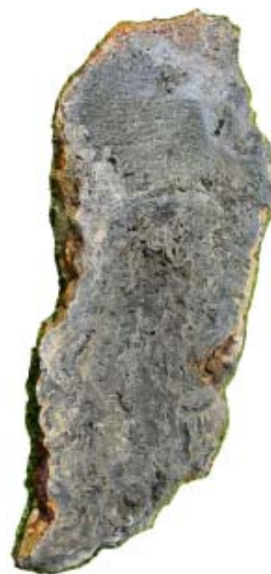
Figure 2. Black smoker chimney containing metalliferous sulphides dated by the ^{210}\text{Pb}/^{226}\text{Ra} method. The length of the chimney is c. 86 cm.
